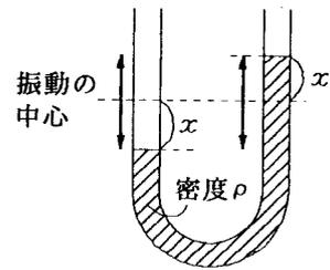
$$\begin{aligned} F &= -2xS\rho g \quad \dots\dots\dots ① \\ &= -2 \times 0.20 \times 0.030 \times 1.0 \times 10^3 \times 9.8 \\ &= -117.6 \approx -120 \text{ [N]} \end{aligned}$$
